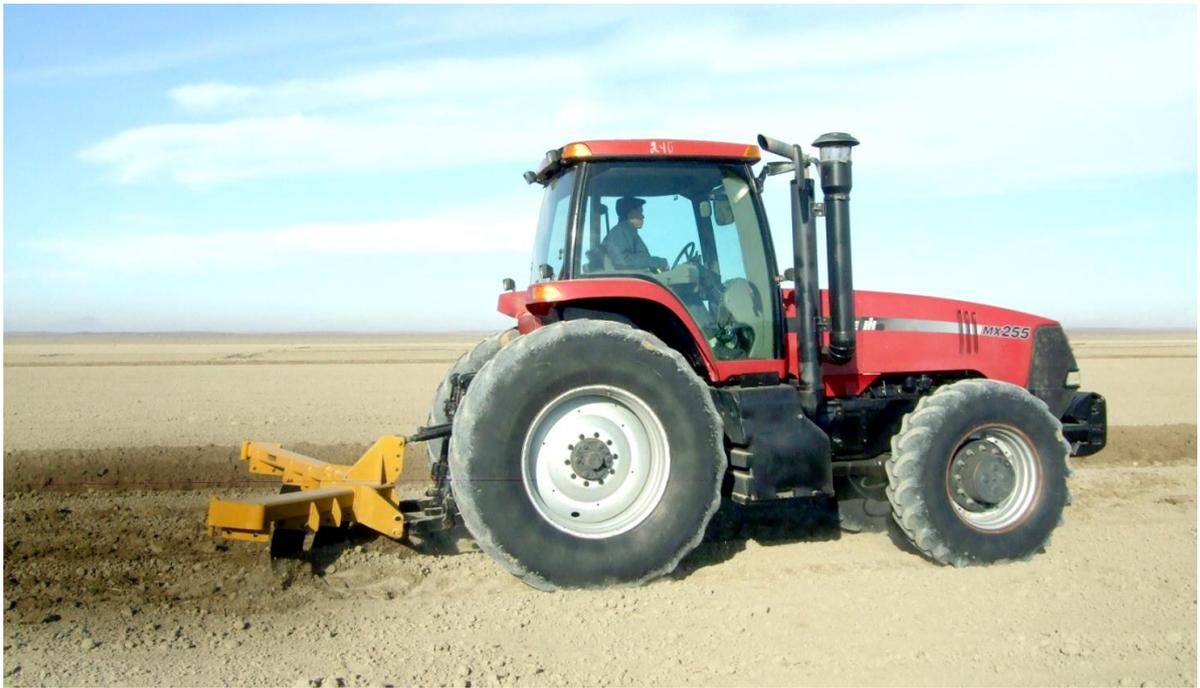
*Figure 4. Deep loosening of the soil*
