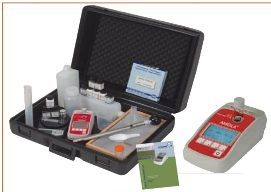
Figure 11.A handy (mobile) device that determines the amount of nutrients in the soil
