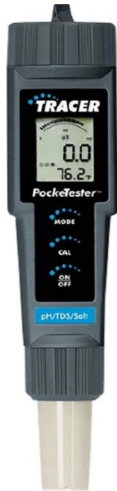
Figure 8. Equipment for determining soil salinity, electrical conductivity and alkalinity
