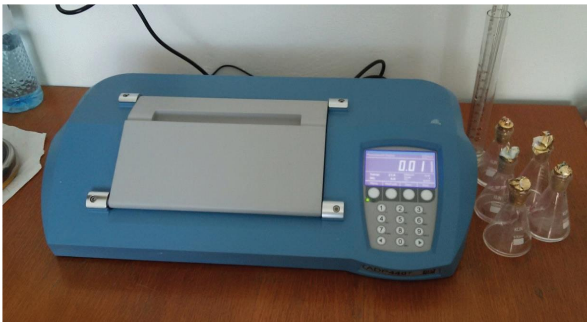
Figure 1. Definition of the absorbent force of the cotton growth in the adp440 plus polarimeter
