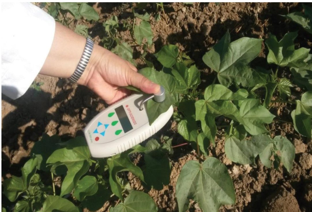
Figure 2. Determination of the amount of chlorophyll on a cotton leaf with a CCM 200 plus
